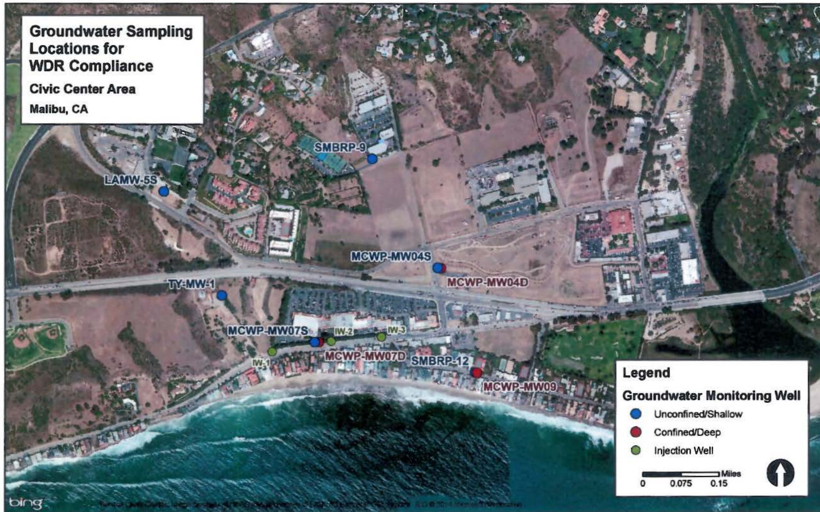
Figure 5 – Locations of Groundwater Monitoring Wells and Injection Wells
