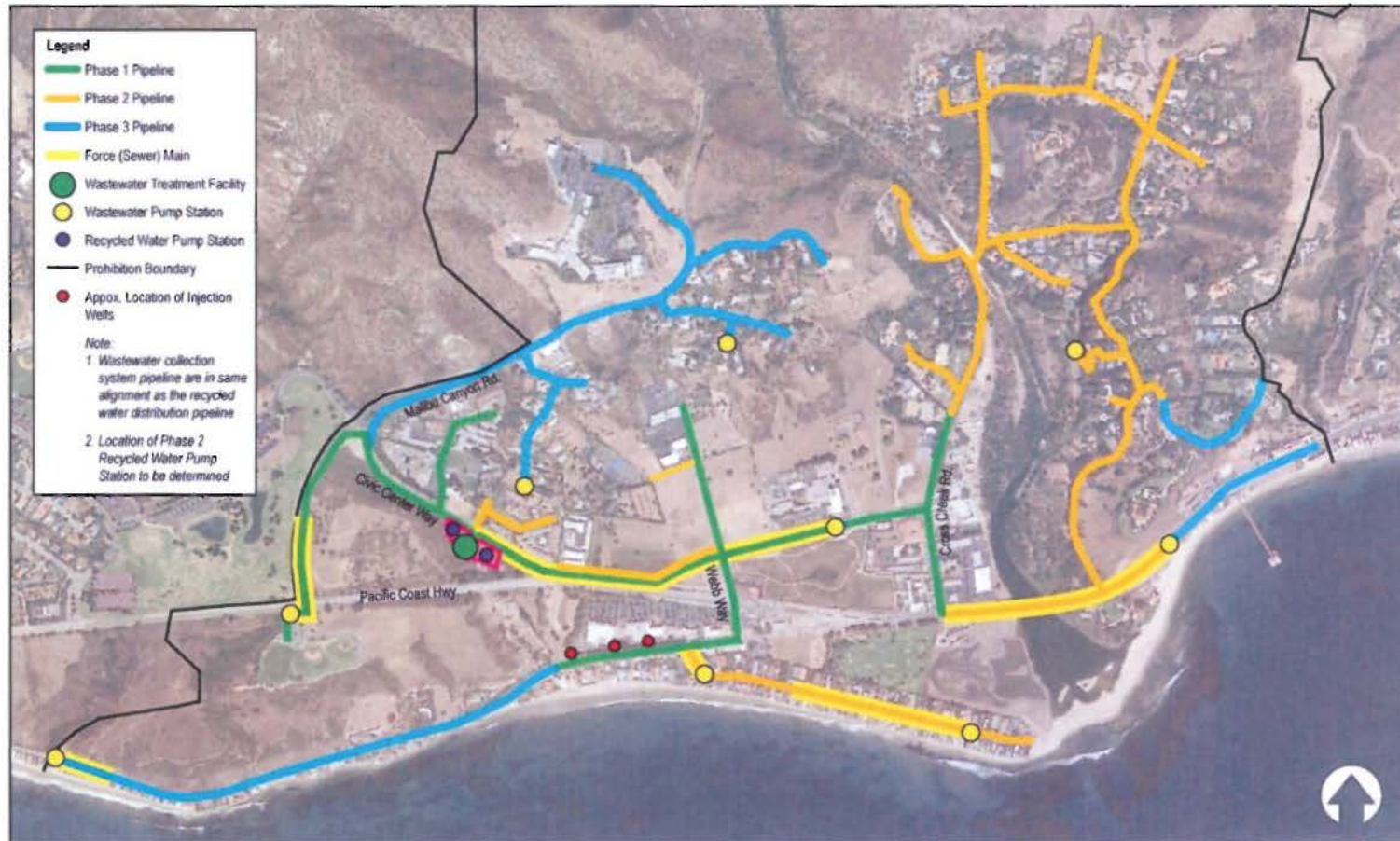
Figure 4 – Locations of Malibu Civic Center Wastewater Treatment Facility, Wastewater Collection and Recycled Water Pipelines, Wastewater and Recycled Water Pump Stations, and Injection Wells
